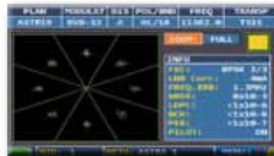
DVB-S2 Constellation 8PSK mod., on the right relative modulation parameters & ISSY
